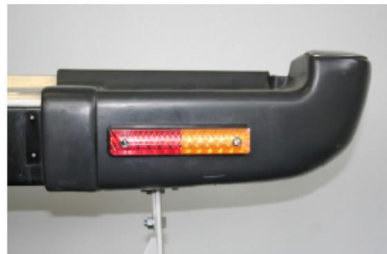
1. Mark bumperette as per photo. Drill two outer holes to 6mm and hole for wiring to 10mm, in centre of two outer holes.
